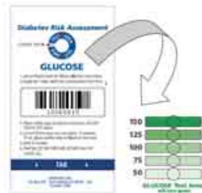
Fig. 6: The ChemCard for glucose is a three-minute determination of blood sugar. A single drop of blood is added to the test area, and the control dot turns red to indicate that sufficient blood exists. After three minutes the tab, which traps the red blood cells, is removed. The shade of green color of the test pad is compared to the reference chart and the best match provides the glucose level in mg/dL. Glucose results 75mg/dL or higher are confirmed with Hemoglobin A1c testing, which is performed on the blood cells trapped in the top layer of the card tab.
