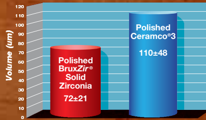
The antagonistic (Stealite balls) wear shows BruxZir Solid Zirconia only with 72±21 micron, which is significantly lower than Ceramco3 (110±48 micron). The University of Tübingen study was run using an eight-chamber Willytec Chewing Simulator at 1.2 million cycles.
